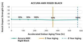
**OUTDOOR STABILITY:** Tested per ASTM G154 standard method.
